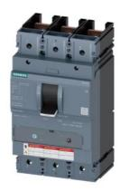
circuit breaker 3VA5 UL frame 400 breaking capacity class M 35kA @ 480 V 3-pole, line protection TM230, FTAM, In=350A without overload protection Ir=350A fixed short circuit protection Ii=5...10 x In w/o connection
