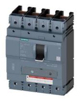
circuit breaker 3VA5 UL frame 400 breaking capacity class C 100kA @ 480 V 4-pole, line protection TM240, ATAM, In=300A overload protection Ir=210A ...300A short circuit protection Ii=5...10 x In neutral unprotected w/o connection
