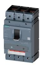
circuit breaker 3VA5 UL frame 400 breaking capacity class C 100kA @ 480 V 3-pole, line protection TM240, ATAM, In=300A overload protection Ir=240A ...300A short circuit protection Ii=5...10 x In nut keeper kit on both sides
