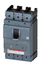
circuit breaker 3VA5 UL frame 400 breaking capacity class C 100kA @ 480 V 3-pole, line protection TM240, ATAM, In=300A overload protection Ir=210A ...300A short circuit protection Ii=5...10 x In w/o connection
