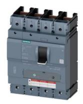
circuit breaker 3VA5 UL frame 400 breaking capacity class C 100kA @ 480 V 4-pole, line protection TM230, FTAM, In=300A overload protection Ir=300A fixed short circuit protection li=5...10 x In neutral unprotected w/o connection
