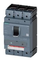
circuit breaker 3VA5 UL frame 400 breaking capacity class C 100kA @ 480 V 3-pole, line protection TM230, FTAM, In=300A overload protection Ir=300A fixed short circuit protection li=5...10 x In Al-lug, line and load side
