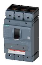
circuit breaker 3VA5 UL frame 400 breaking capacity class C 100kA @ 480 V 3-pole, line protection TM230, FTAM, In=300A overload protection Ir=300A fixed short circuit protection li=5...10 x In nut keeper kit on both sides
