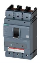
circuit breaker 3VA5 UL frame 400 breaking capacity class C 100kA @ 480 V 3-pole, line protection TM230, FTAM, In=300A overload protection Ir=300A fixed short circuit protection li=5...10 x In w/o connection
