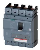
circuit breaker 3VA5 UL frame 400 breaking capacity class M 35kA @ 480 V 4-pole, line protection TM230, FTAM, In=300A without overload protection Ir=300A fixed short circuit protection Ii=5...10 x In neutral protection 1 w/o connection
