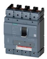
circuit breaker 3VA5 UL frame 400 breaking capacity class C 100kA @ 480 V 4-pole, line protection TM240, ATAM, In=250A overload protection Ir=175A ...250A short circuit protection Ii=5...10 x In neutral unprotected w/o connection
