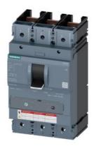
circuit breaker 3VA5 UL frame 400 breaking capacity class H 65kA @ 480 V 3-pole, line protection TM240, ATAM, In=250A without overload protection Ir=175A ...250A short circuit protection Ii=5...10 x In w/o connection
