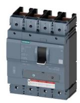
circuit breaker 3VA5 UL frame 400 breaking capacity class C 100kA @ 480 V 4-pole, line protection TM240, ATAM, In=225A overload protection Ir=157,5A ...225A short circuit protection li=5...10 x In neutral protection 1 w/o connection
