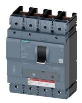
circuit breaker 3VA5 UL frame 400 breaking capacity class C 100kA @ 480 V 4-pole, line protection TM240, ATAM, In=225A overload protection Ir=157,5A ...225A short circuit protection Ii=5...10 x In neutral unprotected w/o connection
