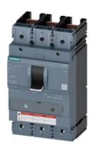
circuit breaker 3VA5 UL frame 400 breaking capacity class C 100kA @ 480 V 3-pole, line protection TM240, ATAM, In=225A overload protection Ir=157,5A ...225A short circuit protection Ii=5...10 x In w/o connection
