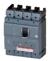
circuit breaker 3VA5 UL frame 400 breaking capacity class C 100kA @ 480 V 4-pole, line protection TM230, FTAM, In=225A overload protection Ir=225A fixed short circuit protection li=5...10 x In neutral unprotected w/o connection
