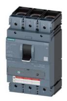
circuit breaker 3VA5 UL frame 400 breaking capacity class C 100kA @ 480 V 3-pole, line protection TM230, FTAM, In=225A overload protection Ir=225A fixed short circuit protection Ii=5...10 x In Al-lug, line and load side
