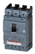
circuit breaker 3VA5 UL frame 400 breaking capacity class C 100kA @ 480 V 3-pole, line protection TM230, FTAM, In=225A overload protection Ir=225A fixed short circuit protection li=5...10 x In w/o connection
