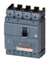
circuit breaker 3VA5 UL frame 400 breaking capacity class H 65kA @ 480 V 4pole, line protection TM240, ATAM, In=225A without overload protection Ir=157,5A ...225A short circuit protection Ii=5...10 x In neutral protection 1 w/o connection
