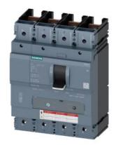
circuit breaker 3VA5 UL frame 400 breaking capacity class H 65kA @ 480 V 4-pole, line protection TM240, ATAM, In=225A without overload protection Ir=157,5A ...225A short circuit protection li=5...10 x In neutral unprotected w/o connection
