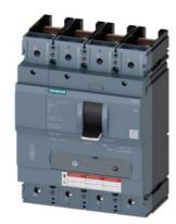
circuit breaker 3VA5 UL frame 400 breaking capacity class H 65kA @ 480 V 4-pole, line protection TM230, FTAM, In=225A without overload protection Ir=225A fixed short circuit protection Ii=5...10 x In neutral unprotected w/o connection
