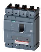
circuit breaker 3VA5 UL frame 400 breaking capacity class M 35kA @ 480 V 4-pole, line protection TM230, FTAM, In=225A without overload protection Ir=225A fixed short circuit protection Ii=5...10 x In neutral protection 1 w/o connection
