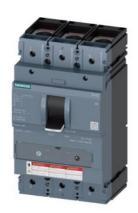
circuit breaker 3VA5 UL frame 400 breaking capacity class C 100kA @ 480 V 3-pole, line protection TM240, ATAM, In=200A overload protection Ir=160A ...200A short circuit protection Ii=5...10 x In Al-lug, line and load side
