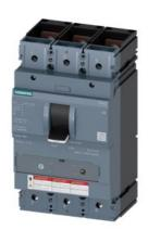
circuit breaker 3VA5 UL frame 400 breaking capacity class C 100kA @ 480 V 3-pole, line protection TM240, ATAM, In=200A overload protection Ir=160A ...200A short circuit protection Ii=5...10 x In nut keeper kit on both sides
