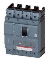
circuit breaker 3VA5 UL frame 400 breaking capacity class C 100kA @ 480 V 4-pole, line protection TM230, FTAM, In=200A overload protection Ir=200A fixed short circuit protection li=5...10 x In neutral unprotected w/o connection
