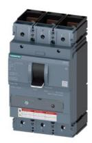
circuit breaker 3VA5 UL frame 400 breaking capacity class C 100kA @ 480 V 3-pole, line protection TM230, FTAM, In=200A overload protection Ir=200A fixed short circuit protection li=5...10 x In nut keeper kit on both sides
