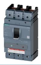
circuit breaker 3VA5 UL frame 400 breaking capacity class C 100kA @ 480 V 3-pole, line protection TM230, FTAM, In=200A overload protection Ir=200A fixed short circuit protection li=5...10 x In w/o connection
