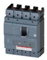
circuit breaker 3VA5 UL frame 400 breaking capacity class H 65kA @ 480 V 4-pole, line protection TM240, ATAM, In=200A without overload protection Ir=140A ...200A short circuit protection Ii=5...10 x In neutral unprotected w/o connection
