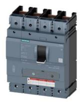
circuit breaker 3VA5 UL frame 400 breaking capacity class H 65kA @ 480 V 4-pole, line protection TM230, FTAM, In=200A without overload protection Ir=200A fixed short circuit protection Ii=5...10 x In neutral unprotected w/o connection
