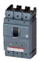
circuit breaker 3VA5 UL frame 400 breaking capacity class M 35kA @ 480 V 3-pole, line protection TM240, ATAM, In=200A without overload protection Ir=140A ...200A short circuit protection Ii=5...10 x In w/o connection
