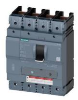
circuit breaker 3VA5 UL frame 400 breaking capacity class M 35kA @ 480 V 4-pole, line protection TM230, FTAM, In=200A without overload protection Ir=200A fixed short circuit protection Ii=5...10 x In neutral unprotected w/o connection
