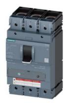
circuit breaker 3VA5 UL frame 400 breaking capacity class M 35kA @ 480 V 3-pole, line protection TM230, FTAM, In=200A overload protection Ir=200A fixed short circuit protection Ii=5...10 x In Al-lug, line and load side
