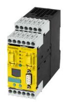
DP/AS-Interface F-Link. gateway PROFIBUS DP/AS-i for safety-oriented data transmission from ASIsafe to PROFIBUS-DP-PROFIsafe. Master profile M3/M4 according to AS-i specification V3.0. degree of protection IP20. screw terminals
