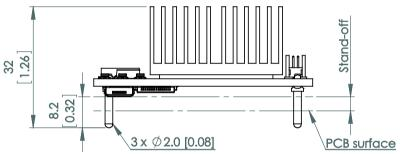
Weight: Typical 54g All dimensions in mm [inch] Tolerances unless specified ±0.25 [0.01]
