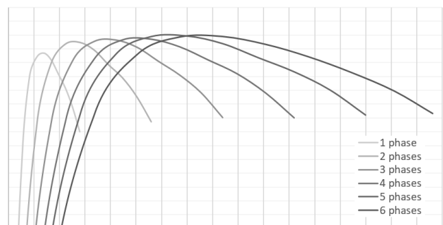
Illustration of efficiency vs load and number of active phases.
