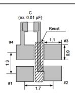
To maintain stable operation, provide a 0.01uF to 0.1uF by-pass capacitor at a location as near as possible to the power source terminal of the crystal product (between Vcc - GND).
