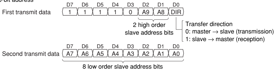
Figure 20.5.2 Transmit Data to Specify Slave Address and Data Direction
