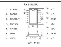
The metal case inside of the molding compound may be exposed on the top or bottom of this product.
