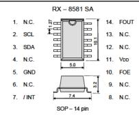
The metal case inside of the molding compound may be exposed on the top or bottom of this product. This purely cosmetic and does not have any effect on quality, reliability or electrical speci
