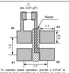
To maintain stable operation, provide a 0.01uF to 0.1uF by-pass capacitor at a location as near as possible to the power source terminal of the crystal product (between Vcc - GND).
