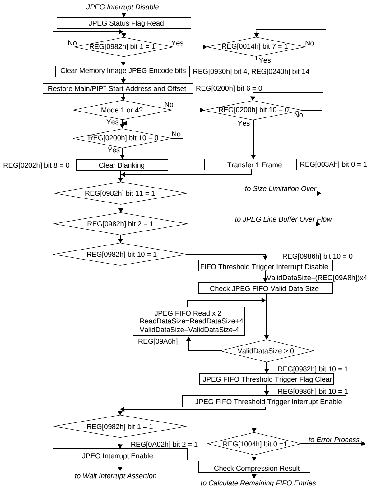
Figure 14-8: Memory Image JPEG Encoding Process (3 of 4)
