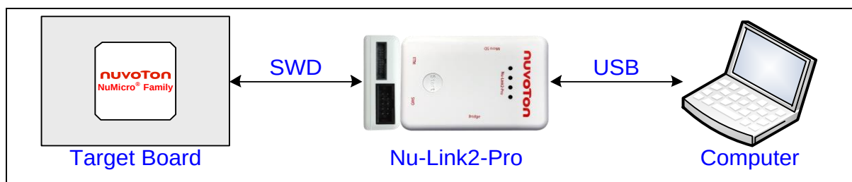
Figure 5.1-1 Nu-Link2-Pro Connection Diagram
