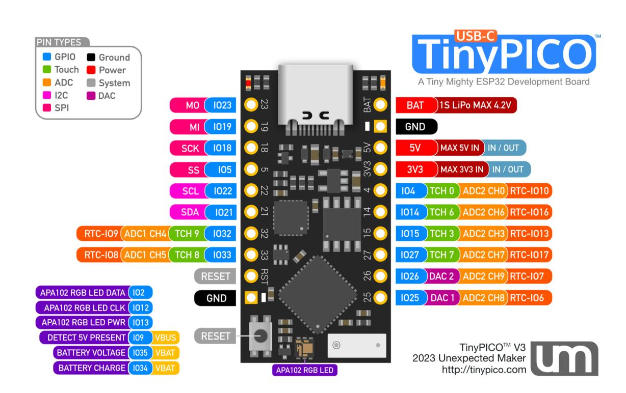
35mm x 17.8mm **Board Dimensions Max Thickness** 4.3mm at the USB-C end
