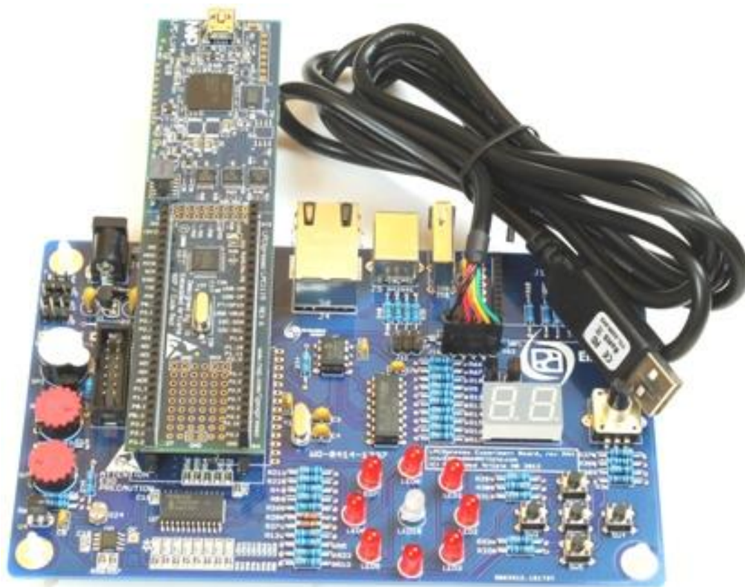
Figure 59 – LPCXpresso Experiment Kit PCB with UART-to-USB Cable
