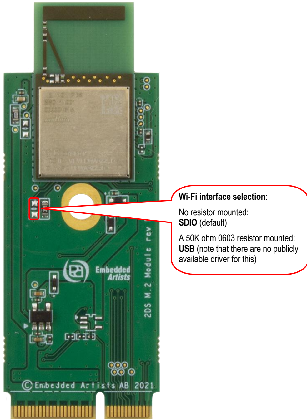
Figure 4 – 2DS M.2 Module Wi-Fi Interface Selector
