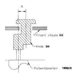
3. Regarding the operating of the lever. please consider the above mentioned, and make sure nothing is wrong with the operation under installing in your appliance that you plan to use our products actually. Knob assembly on the lever and functioning the lever to be performed under the condition of P.C.B. without worp.
