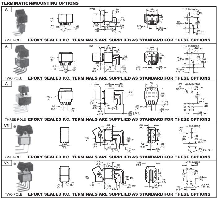
1 The V5 option is available in Three and Four Pole Circuits
