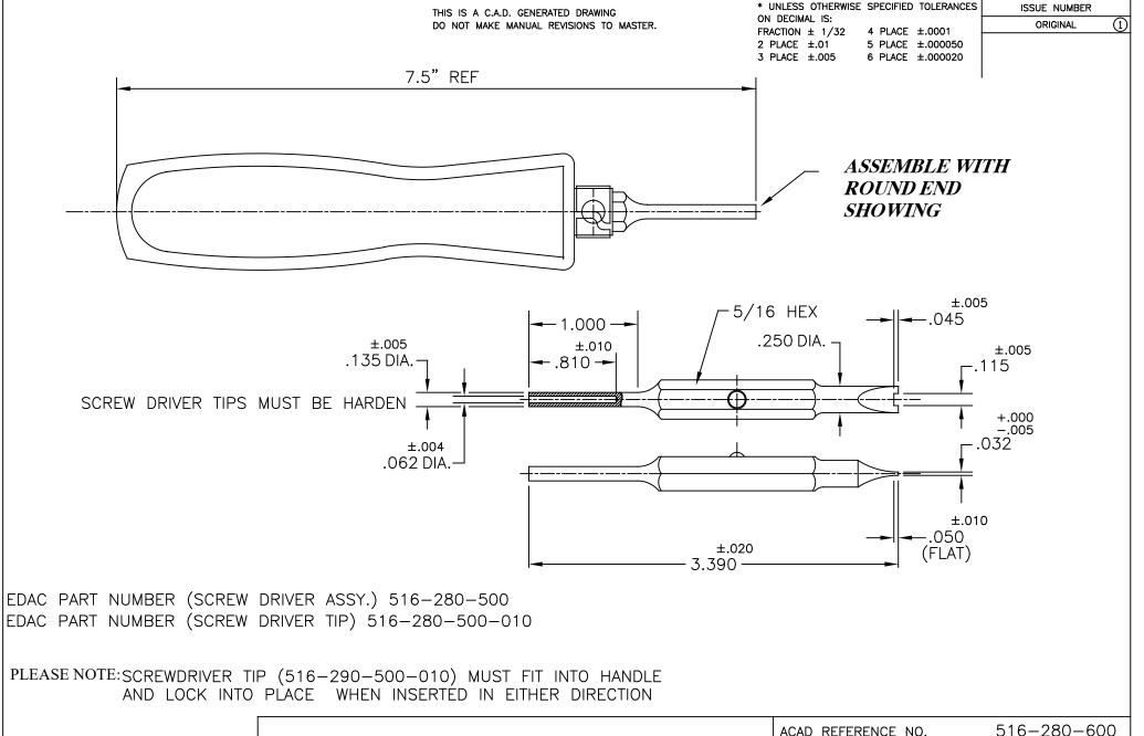
516-280-600 ACAD REFERENCE NO. DATE: SEP.24/11 DRAWN: N.SONDH 516 CONTACT INSERTION TOOL CHECKED: DATE: SCALE: (IN C.A.D. 1:1) SHEET 1 OF 1 THESE DRAWINGS AND SPECIFICATIONS EDAC INC ARE THE PROPERTY OF EDAC INC., AND TORONTO, ONTARIO SHALL NOT BE REPRODUCED, OR COPIED DRAWING NUMBER **ISSUE** OR USED AS THE BASIS FOR THE CANADA MANUFACTURE OR SALE OF APPARATUS 516-280-600 YOUR CONNECTION TO QUALITY & SERVICE WITHOUT WRITTEN PERMISSION.
