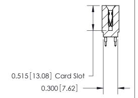
745 Series Ultra-Mate Card Edge Connector - Press Fit ACAD REFERENCE NO. Part Number: 745-074-560-201
