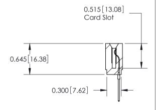
737 Series Ultra-Mate Card Edge Connector - Press Fit ACAD REFERENCE (CITION - FACAD REFERENCE ( Part Number: 737-016-545-101 THESE DRAWINGS AND SPECIFICATIONS
