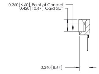
726 Series Ultra-Mate Card Edge Connector - Press Fit Part Number: 726-025-540-101 **EDAC INC** THESE DRAWINGS AND SPECIFICATIONS ARE THE PROPERTY OF EDAC INC.,AND TORONTO, ONTARIO SHALL NOT BE REPRODUCED, OR COPIED CANADA
